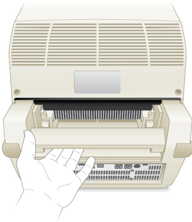
8. If you have not done so, insert one end of the supplied power cable into the base of the thermal cycler and the other end into an appropriate electrical outlet.
