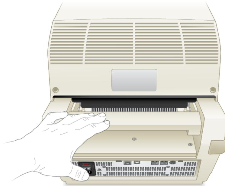
2. Carefully lift the reaction module out of the bay using the handle indents on each side.
