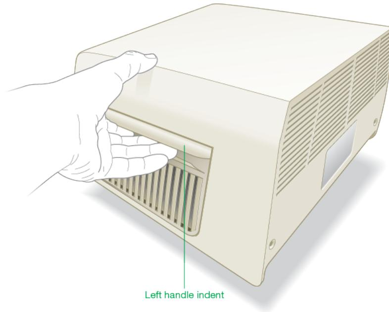
6. With its lid lever pointing toward the front, insert the reaction module into the reaction module bay, leaving about 2 cm of space in front of the thermal cycler.
