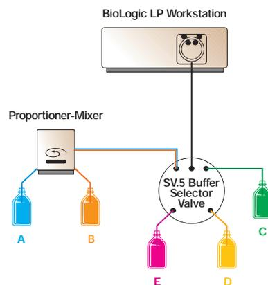
**Buffer plumbing scheme.** A. Binding buffer (20 mM Tris base, 0.5 M NaCl, 5 mM imidazole, pH 7.8) containing 8 M urea. B. Binding buffer (20 mM Tris base, 0.5 M NaCl, 5 mM imidazole, pH 7.8). C. Wash buffer (20 mM Tris base, 0.5 M NaCl, 20 mM imidazole, pH 7.8) containing 8 M urea. D. Elution buffer (20 mM Tris base, 0.5 M NaCl, 0.3 M imidazole, pH 7.8). E. Protein sample.
