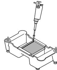
6. Secure the lid on the gel box. The lid will attach to the base in only one orientation: red to red and black to black. Connect the electrical leads to the power supply.
