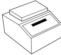
6. When all of the PCR samples are in the thermal cycler, the teacher will begin the PCR reaction. The reaction will undergo 40 cycles of amplification, which will take approximately 3 hours.
