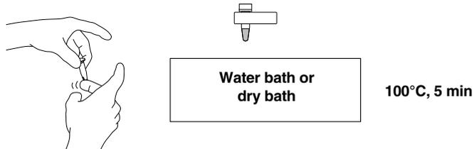
5. Remove your tube from the boiling water bath and shake or vortex to resuspend the contents. Pellet the matrix by spinning at 6,000 x g for 5 minutes (or 2,000 x g for 10 minutes).
