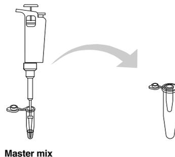
5. Remove your PCR tube from the PCR capless adapter tube and place the PCR tube in the thermal cycler.
