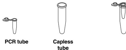
3. Transfer 20  $\mu$ l of your DNA template from the supernatant in your screwcap tube into the bottom of the PCR tube. **Do not transfer any of the matrix beads into the PCR reaction because they will inhibit the PCR reaction.**
