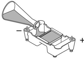
5. Using a clean tip for each sample, load the samples into the 8 wells of the gel in the following order:
