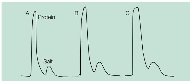
**Fig. 2. Effect of sample volume on desalting.** A, 1 ml sample (20% of gel volume) containing 1.3 mg/ml BSA, 2 mg/ml NaNO<sub>3</sub> on a 1.0 x 10 cm Econo-Column chromatography column containing 5 ml Bio-Gel P-6DG at a flow rate of 30 ml/hr. B, 1.5 ml sample (30% of gel volume); all other conditions as in A. C, 2.0 ml sample (40% of gel volume); all other conditions as in A.
