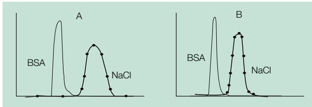
**Fig. 1. Desalting of BSA on Bio-Gel P-6DG gel using conditions outlined in Table 1.** A, 1.5 ml sample containing 1.25 mg/ml BSA in 2 M NaCl run on a 1.0 x 10 cm Econo-Column® chromatography column containing 6 ml Bio-Gel P-6DG at a flow rate of 39 ml/hr (gravity flow). B, 10 ml sample containing 2 mg/ml BSA in 2 M NaCl run on a 2.5 x 10 cm Econo-Column chromatography column containing 40 ml Bio-Gel P-6DG at a flow rate of 120 ml/hr (gravity flow).
