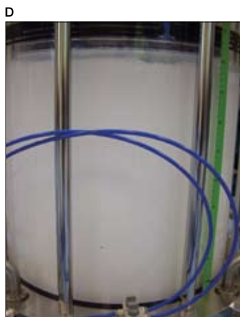
Fig. 3. Bio-Rad InPlace column repacking. A , initiation of upflow at 100 cm/hr while the top piston was raised; B , end of upflow and bed resuspension in PBS at 40% (v/v); C , fully resuspended bed; D , sparging with air was performed for >10 min to bring the suspension to homogeneity while preventing shearing of CHT.
