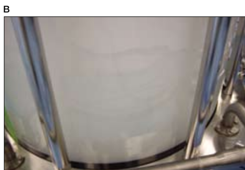
Fig. 2. Fully packed 45 cm Bio-Rad InPlace column. CHT Type I support, 40 \mu\text{m} , was hydrated and packed in a 40% (v/v) suspension in PBS.
