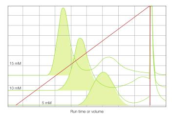
Fig. 3. Elution of protein A-purified IgG1 from CHT ceramic hydroxyapatite. A 40 column volume linear gradient to 1.0 M NaCl (—) at three constant phosphate concentrations is shown. Data indicate a trend of decreasing aggregate resolution with increasing phosphate concentration.
