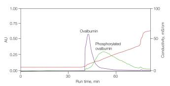
Fig. 4. Resolution of ovalbumin from its phosphorylated counterpart using CHT ceramic hydroxyapatite. Note the longer retention time for phosphorylated ovalbumin. Increasing the phosphate content of ovalbumin by conjugation of phosphoserine enhanced retention on CHT. Red trace shows conductivity (phosphate gradient).
