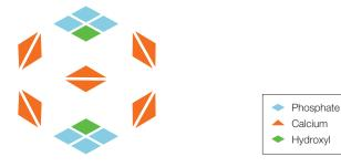
Fig. 1. Crystal structure of CHT ceramic hydroxyapatite,  $Ca_{10}(PO_4)_6(OH)_2$ . Each molecule consists of five positively charged calcium pairs (C-sites); two phosphate triplets (P-sites), each with six negatively charged oxygen atoms; and two hydroxyl residues.
