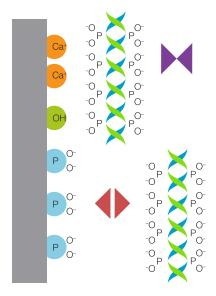
Fig. 6. Interaction of DNA with CHT ceramic hydroxyapatite. Note the electrostatic repulsion between CHT P-sites and the phosphate backbone of DNA, and the interaction of that backbone with the C-sites and hydroxyl groups. (Symbols same as in Figure 2.)
