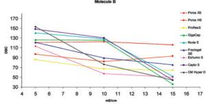
The comparisons of the two molecules shows that there is a big difference between how the molecules behave with different resins and at different conductivities. Selecting a single resin based on DBC as a first pass criteria, will have to be expanded to measuring product quality attributes as well.
