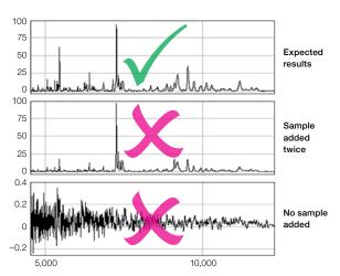
Spectra examples, as included in the manual, help to identify possible technical errors that can cause problems. Data illustrate the results of an error made in the number of additions of sample to the CM10 array during the binding step.
