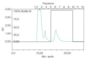
Fig. 3. Purification of a 45 kD histidine-tagged protein on a Nuvia IMAC Column. E. coli extract (2 ml) was loaded on a 0.46 x 5 cm column pre-equilibrated with 50 mM Na<sub>2</sub>PO<sub>4</sub>, 10 mM imidazole, and 300 mM NaCl, pH 7.5 (buffer A). The target protein was eluted with 10 CV 50 mM Na<sub>3</sub>PO<sub>4</sub>, 125 mM imidazole, 300 mM NaCl, pH 7.5 (buffer B). Column chromatography was monitored at OD 280. A<sub>280</sub> (--); %B (--). AU, absorbance units.
