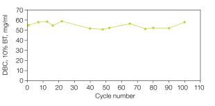
Fig. 6. Reusability of Nuvia IMAC Resin. A 45 kD histidine-tagged protein was loaded onto a 0.5 x 5.1 cm column packed with Nuvia IMAC with a compression factor of 1.25. The column was run at 300 cm/hr. The binding buffer was 50 mM sodium phosphate, 5 mM imidazole, and 300 mM NaCl (pH 7.5) and the elution buffer contained 250 mM imidazole. Solutions for column regeneration are listed in Table 1.
