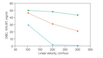
Fig. 1. DBC vs. flow velocity of Nuvia IMAC Resin. Comparison of DBCs between Nuvia IMAC (•), agarose IMAC resin A (=), and agarose IMAC resin B (▲). The resins were packed into 1 ml columns (0.5 x 5 cm). A 45 kD histidine-tagged protein (1.2 mg/ml) in 50 mM sodium phosphate, 5 mM imidazole, 300 mM NaCl (pH 7.5) was loaded onto each column until 10% breakthrough (BT) was observed.
