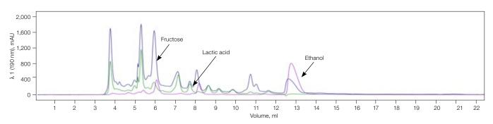
Fig. 3. Chromatogram of a primary fermentation sample. Fructose, 190 nm trace (-); lactic acid, 210 nm trace (-); ethanol, RI detector trace (-).
