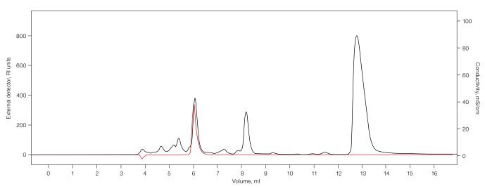
Fig. 6. ChromLab Software evaluation of RI detector data. Overlay chromatograms of a reference fructose solution (--) and secondary fermentation wine sample (--).
