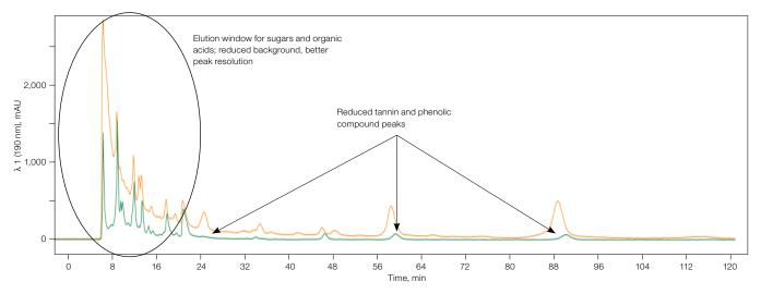
Fig. 2. Treatment of a sample with activated charcoal to remove background interference. Comparison of an untreated wine sample (--) and the sample treated with activated charcoal (--) at 190 nm.
