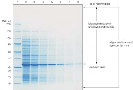
Fig. 1. Example showing MW determination of an unknown protein. Lane 1, 10 µl of Precision Plus Protein™ unstained standards; lanes 2–8, a dilution series of an *E. coli* lysate containing a hypothetical unknown protein (GFP). Proteins were separated by SDS-PAGE in a Criterion™ 4–20% Tris-HCl Gel and stained with Bio-Safe Coomassie stain. Gel shown is the actual size.
