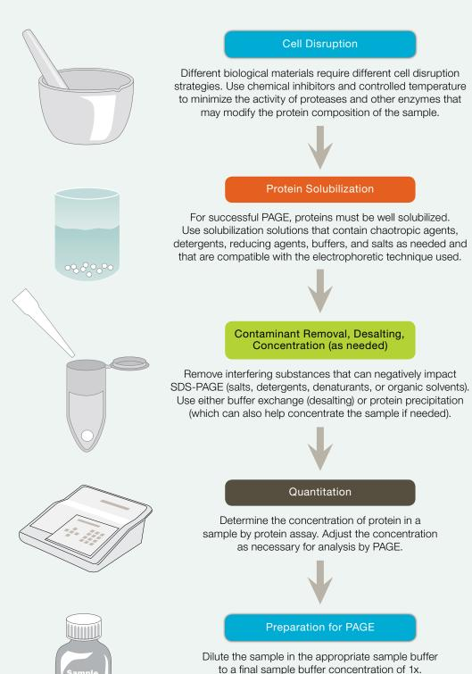
Fig. 3.1. Protein sample preparation workflow.
