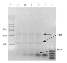
**Fig. 5. Agarose gel electrophoresis of RNA samples containing tRNA.** Mouse brain total RNA samples (200 ng) were spiked with tRNA and then separated by horizontal electrophoresis on a 1% ReadyAgarose gel. Lane 1, 1 kb DNA ladder; lanes 2–5, total RNA containing 0, 20 ng, 40 ng, and 100 ng tRNA, respectively; lane 6, 100 ng tRNA; lane 7, 100 bp DNA ladder.
