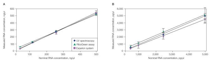
Fig. 1. Linear dynamic range of RNA quantitation. Mouse skin total RNA samples at the concentrations indicated were analyzed using UV spectroscopy, the RiboGreen assay, or the Experion system, and the measured concentration obtained was plotted as a function of the expected (nominal) sample concentration. A, analysis of nanogram levels of total RNA; B, analysis of picogram levels of total RNA.
