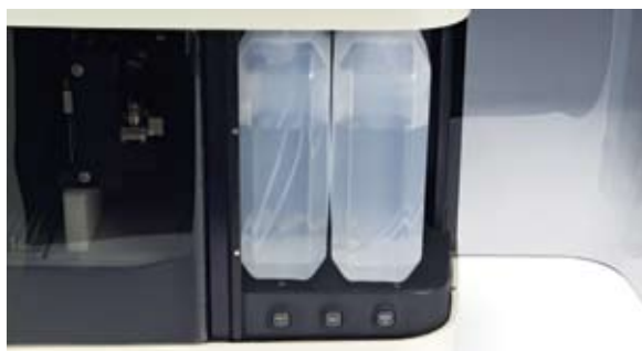
Buffer compartment holds two 2 L autoclavable bottles.
