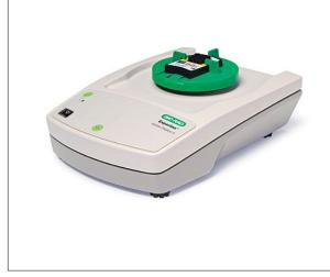
Electrode manifold with 16 high-quality platinum pins for reproducible runs
