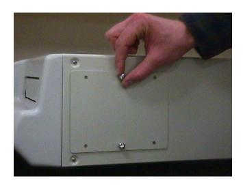
2. Loosen thumbscrews on side panel and remove panel.
