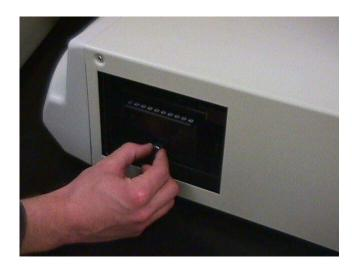
3. Remove thumbscrew holding filter magazine in place.
