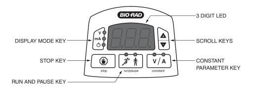
Fig. 3. Front Panel.
