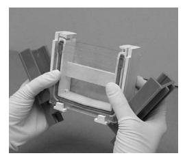
e. The arms of the clamping frame push the short plates up against the notch in the green gasket, creating a leak-proof seal. At this point, the sample wells can be washed out with running buffer, and sample can be loaded.
