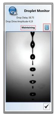
Fig. 41. Droplet Monitor window with status and recalculate button highlighted.
