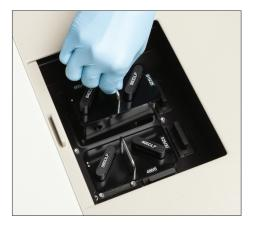
Fig. 69. Lifting an optical filter block.
