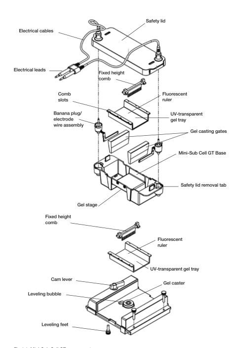
Fig.1.1. Mini-Sub Cell GT components.
