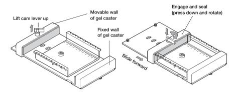
Fig. 2.1. Sealing the UVTP tray for gel casting.
