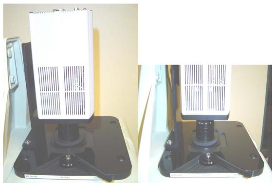
Make sure that the lens is seated properly on the gasket in the adapter.
