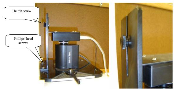
Closeup of Gel Doc XR camera mounted with thumb screw
