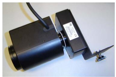
Gel Doc XR camera with bracket, MZL, and thumb screw
