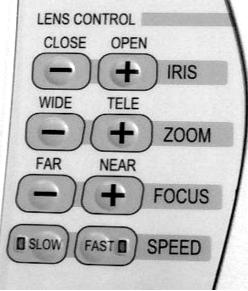
Membrane touch pad – Lens control section
