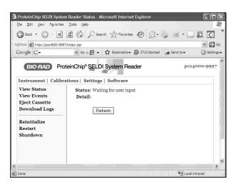
Select Calibrations > Automatic Detector Gain. The Detector Gain page opens. Check that Automatic and NOT manual is selected.
