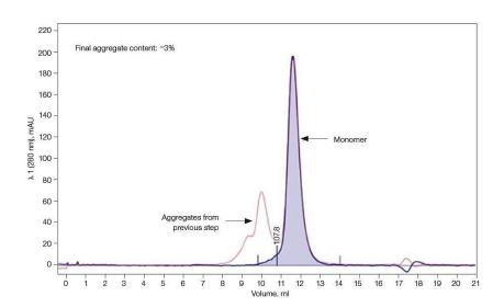
Figure 3. SEC analysis of mAb **S eluted from CHT XT.** SEC showing the level of mAb S aggregates in the eluate from CHT XT. OD 280 (-)
