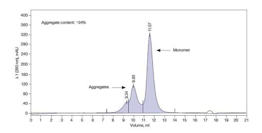
Figure 1. SEC analysis of mAb S eluted from **UNOsphere SuprA.** SEC showing the level of mAb S aggregates in the eluate from UNOsphere SUPrA. This will be the load on CHT XT. OD 280 (-)
