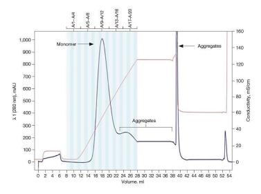
Figure 2. Elution of mAb S monomers from a CHT XT column. The blue vertical bands represent where samples were collected. Fractions 10 to 14 were pooled. OD 280 (purple) %B (red).
