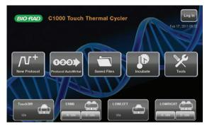
Multi-instrument control. The C1000 Touch Cycler can control multiple thermal cyclers using a single interface.
