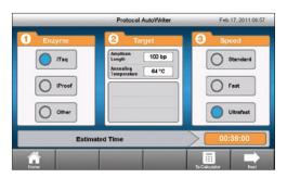
Quick and easy protocol programming. The protocol autowriter in the cycler's onboard software can automatically suggest a fast temperature protocol based on input parameters. Suggested protocol is based on standard PCR guidelines, with hot-start, initial denaturation, annealing, and extension steps. Further reductions of run times are achieved by minimizing the number of steps and cycles, incubation times, and temperature differentials.
