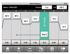
Intuitive graphical programming. The thermal cycler's onboard software displays an editable thermal profile of the PCR protocol, making it easy to create and run new protocols.
