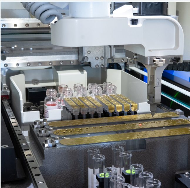
IH-LISS rack piercing
