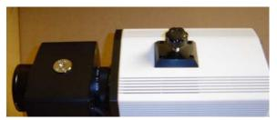
ChemiDoc XRS camera with thumb screw
